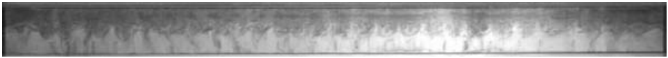
FIGURE 11. Instantaneous photo of dye streaks approximately two periods after start-up for the Re = 1163 and St = 53 . The image was taken looking from above, showing x \in [-\Gamma/2, \Gamma/2] and z \in [-0.9\Lambda/2, 0.9\Lambda/2] , so that only a small portion of the cavity near the two endwalls is missing from the field of view. Dye (dark) was initially deposited along the bottom of the photo.
